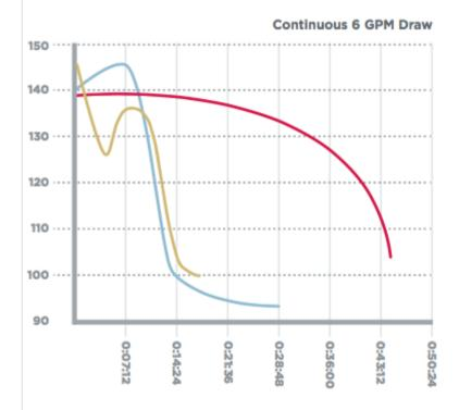
(100°F rise, standard 80-gallon tank vs. high-efficiency 100-gallon tank vs. Demand Duo)
