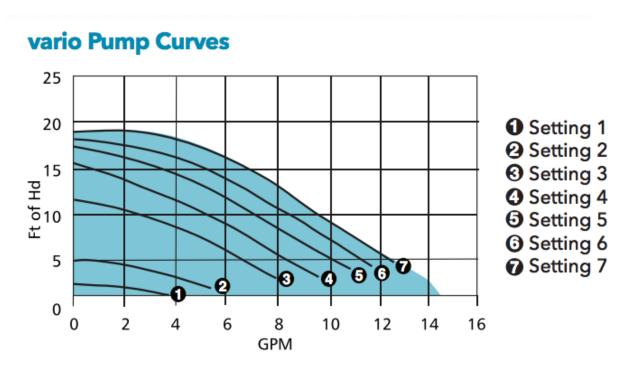
The primary difference in the two models is their control logic. In the vario, constant curve control is employed. This means that the pump follows the natural hydraulic curve and functions much in the same way as a 3-speed circulator pump. However, with the step-less speed dial, you have unlimited speed control of the circulator.
