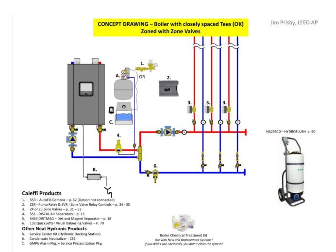
If you're looking for the fastest way to setup a workable primary-secondary circuit, this is a great choice. It will increase the overall volume of your system and you won't break the bank getting it installed. This is a less-than-ideal setup if your zones of heating are very small, as that could cause short-cycling.
