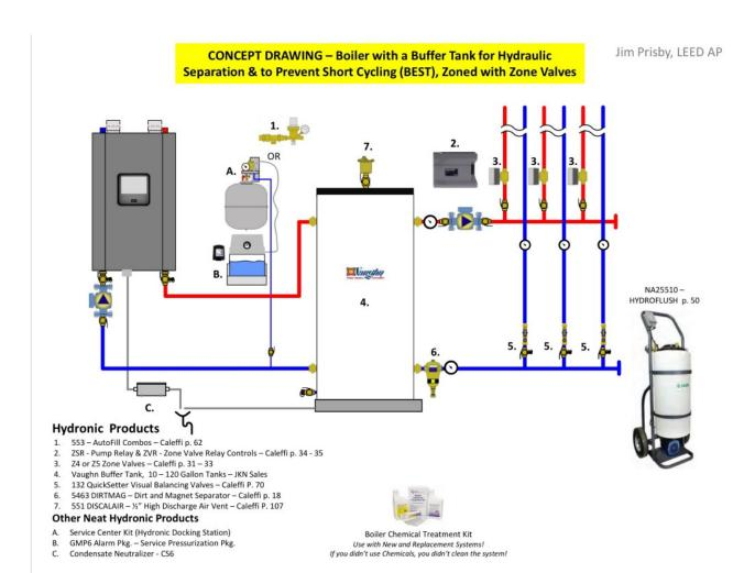
Our final suggestion utilizes the previous application as a base and adds a buffer tank. The tank further increases system volume and system efficiency. It also provides a location for heated water to be stored before being circulated, allowing the additional heat to be spread through your zones without firing the boiler.
