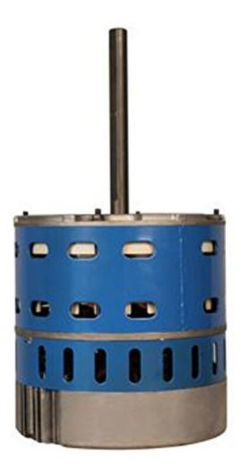
The 10860 and 10861 models can be used for applications between 1/5 HP and 1 HP. Each motor features four speeds and a constant fan mode. There is a handheld programmer available that allows you to adjust the speed between 350 RPM and 1,400 RPM.
