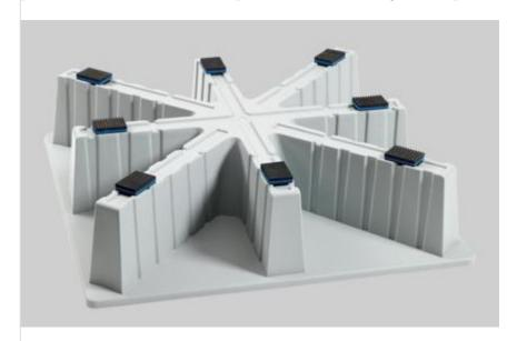
The HP3232-8 is a 32" x 32" condenser pad with eight 8" integral risers. Each riser features an antivibration pad to reduce operational noise. The base of the pad is designed with a slope which diverts condensate from cooling operations or defrost operations away from the equipment. The HP3232-8 is made from durable, environmentally-friendly recycled polypropylene. It is designed to withstand the elements, including UV light, and to last longer than the lifespan of the average heat pump.
